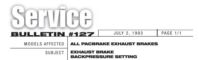
Field reports have indicated some confusion exists between preset exhaust brakes and non preset units. Non-preset exhaust brakes have a tag attached which indicates the unit MUST be road tested to set the brake to the engine manufacturers recommended maximum backpressure as per the Pacbrake application guide.
