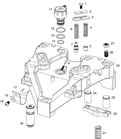
**NOTE:** ALL PARTS SHOWN INTERFACE WTIH DETROIT DIESELS NEW REPLACEMENT INJECTOR. PARTS 19-21 MUST BE PLACED AS AN ASSEMBLY. A RETRO-FIT KIT IS AVAILABLE FOR THIS APPLICATION AND MUST BE INSTALLED IF AN INJECTOR IS BEING REPLACED. SEE SERVICE BULLETIN #154. INJECTOR RETRO-FIT KIT #P63012 WILL UPDATE 3 HOUSINGS.
