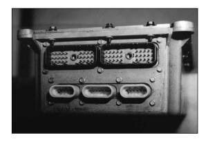
The ECM is mounted on the left side of the engine block, and #508 wire will be the uppermost one closest to the engine.
