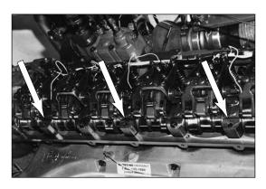
Place a special hardened washer on each of the nine Pacbrake 12 pt. flange screws.
