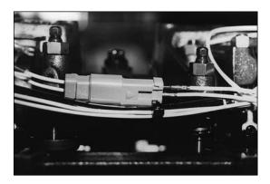
This connector is polarized and may now be parted and reconnected without losing correct brake sequencing.
