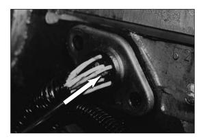
Insert both wires of the Pacbrake 'through head harness' through the grommet from the outside.
