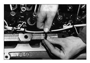
Move to the camshaft side of the engine. Remove the three outboard 12 pt. flange screws holding the camshaft bearing caps in locations #2, 4, and 6, as shown by the arrows.
