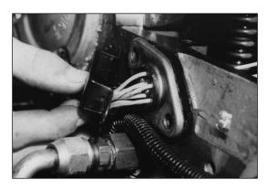
There are four spare holes through the harness grommet which are sealed with plastic plugs. Pulling outward, remove any two of these plugs.
