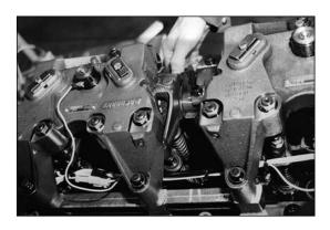
Slave lash may now be adjusted on all cylinders which have clearance between the exhaust rocker adjusting screw and valve stems. Turn the Paclash screw clockwise to establish zero exhaust valve lash. Once zero lash is determined, turn screw an additional 1/4 turn to squeeze out any trapped oil, then back screw out to zero lash.
