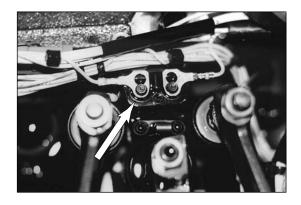
Secure the complete Pacbrake harness to the EUI harness with plastic ties.
