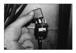
Install on/off switch and three-position switch in dash, conveniently located for the driver.
