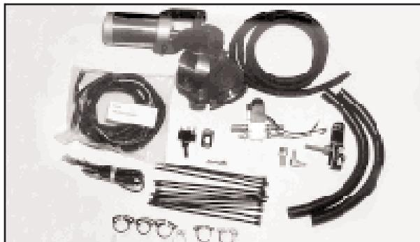
Pacbrake kit C14024 is designed for maximum retarding on your 1998 and newer Dodge 24 valve turbo diesel engine.
