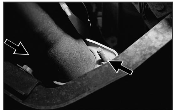
**3** Remove the passenger-side intercooler pipe and remove the engine lifting eye, located by the turbocharger. Remove the turbo outlet V-clamp and move the pipe away from the turbo.
