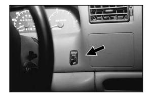
Locate a 12 volt ignition power supply in the harness directly below the steering column (see arrow).
