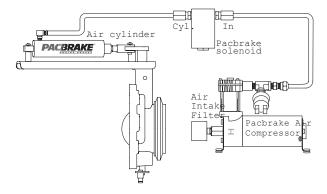
Mount the solenoid to the firewall as shown using the two self-tapping screws provided (it may be easier to drill a pilot hole). Connect the air line from the compressor to the port marked "in" and the port marked "cyl" to the Pacbrake air cylinder.
