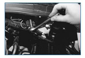
Ford installs a brake pressure applied switch on the front lower side of the master cylinder.
