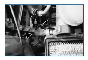
The firewall has a plug which can be removed to insert the harness. If this hole has been used it will be necessary to drill a hole for the harness. Feed the harness through the hole and seal around the loom.
