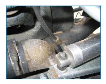
15 Install the 1/4"NPT-1/4" push on barbed hose fitting on to the plastic filter housing. Locate the Blue nylon hose and connect one end to the barbed fitting on the intake filter. Install the compressor air intake filter into the hole located in the radiator support bracket behind the driver side headlight as shown in the photo. Route this line up to the compressor, and connect the other end to the push to connect fitting on the bottom side of the compressor.
