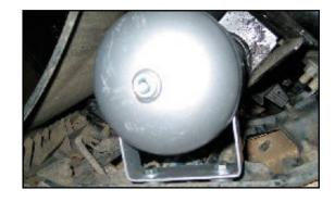
18 Connect the Black nylon airline to the remaining fitting at the compressor. Route it to the top of the air tank. Cut the airline to length with a sharp razor knife. Connect the ¼" airline to either fitting in the tank. Secure the airline away from moving parts and heat sources using the tiestraps provided.
