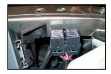
20 Under the hood, route the leg of the Pacbrake wiring harness with the two Weather-Pac connectors to the air compressor. Connect the female connector to the male connector at the compressor and connect the male connector to the female connector at the pressure switch. Secure the harness with the tie-straps provided.
