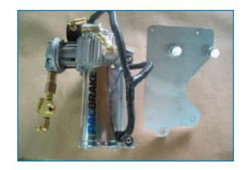
10 Machine screws must be installed as shown in the photo (threaded ends pointing upwards).
