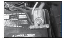
Connect the black wire with the eye terminal to the negative battery terminal or a good chassis ground.
