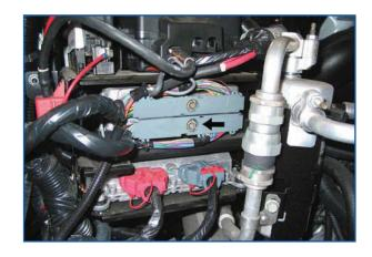
Using the self tapping screw supplied, mount the relay receptacle on the side of the ECM bracket with the wire ends of the relay receptacle pointing down. Install relay. (see arrow on diagram)
