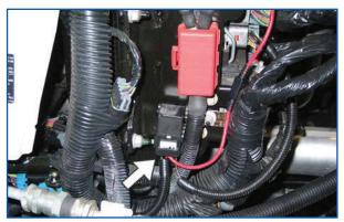
Under the ECM support bracket locate the two weather-pac connectors (see arrows). In the outer 30-pin connector locator the black wire with a white stripe in Pin C7. Cut this wire and T-Tap/splice the Pacbrake RED wire into the factory wire. Crimp the connector to the wire and heat the connector to provide a water tight seal.
