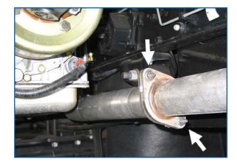
As shown, measure from the exhaust brakes pressure flange to the end of the Pacbrake adapter. Keep in mind the adapter is expanded to fit over the original pipe.
