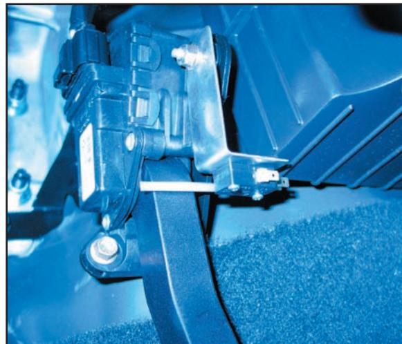
Note: 2005 vehicles equipped with automatic transmissions require the use of C20141 throttle switch group as the engine ECU is not turned on for exhaust braking.
