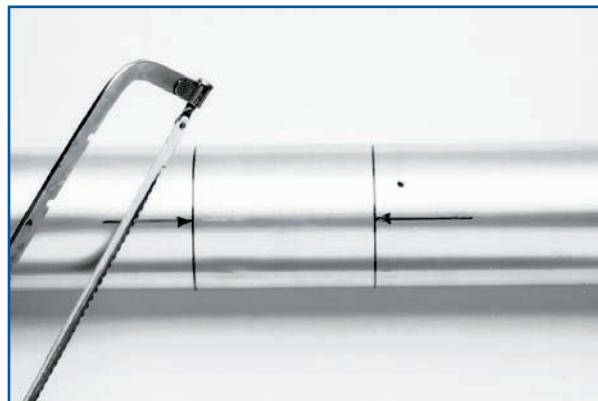
**NOTE:** In some cases, the cutting and welding of exhaust systems can be done without removing the pipe sections from the vehicle.
