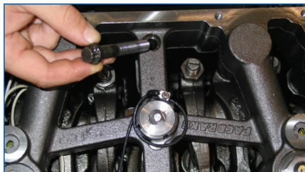
**5** Carefully run the capscrews down evenly in the torque sequence below.
