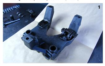
SLAVE PISTON SPRING: Prior to assembly, be sure there are no burrs or sharp edges on the machined surface where the slave piston spring will be secured.
