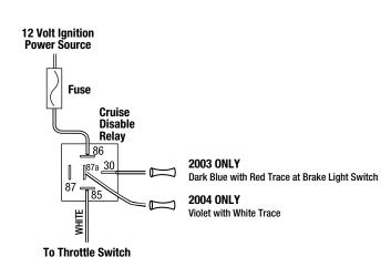
The BLACK wire needs to be routed into the cab, as this wire needs to be connected to the throttle switch in step 2. The WHITE wire originates at the Pacbrake dash switch, route this wire to the throttle switch as it needs to be connected to the throttle switch in step 3.
