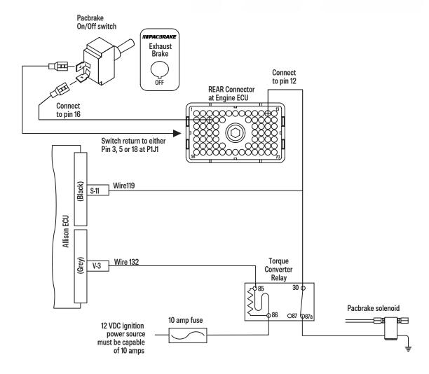
The switch input at J1/P1:16 requires that the "Exhaust Brake Switch" be programmed to "Installed". The parameter "Exhaust Brake Warm-up Configuration" Must be programmed to "Exhaust Brake Only" or "Exhaust Brake & Warm Up".
