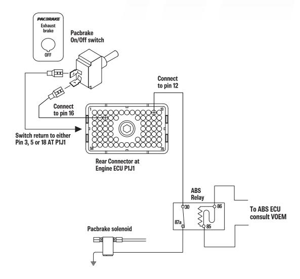
The switch input at J1/P1:16 requires that the "Exhaust Brake Switch" be programmed to "Installed". The parameter "Exhaust Brake Warm-up Configuration" must be programmed to "Exhaust Brake Only" or "Exhaust Brake & Warm Up".
