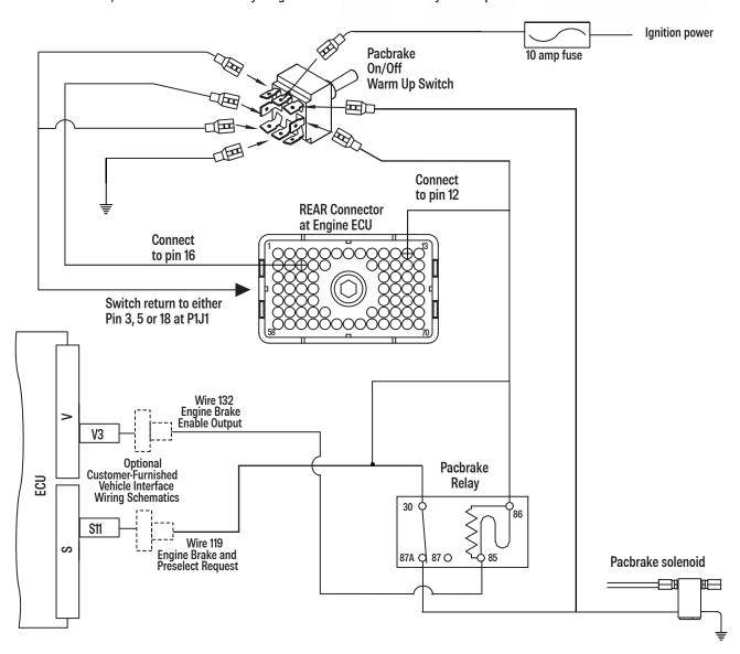
Early 2002 production 3126E engines have the ability to be programmed to allow the exhaust brake to assist the engine in warming up faster in cold weather. Program, customer parameter to "Exhaust Brake and Warm-up" and program warm-up mode IDLE speed to 1100 RPM.
