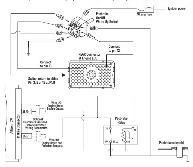
Early 2002 production 3126E engines have the ability to be programmed to allow the exhaust brake to assist the engine in warming up faster in cold weather. Program, customer parameter to "Exhaust Brake and Warm-up" and program warm-up mode IDLE speed to 1100 RPM.
