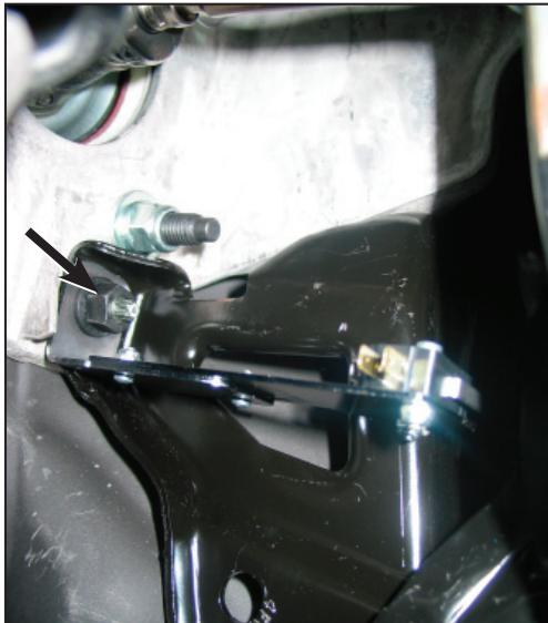
The engines ECM has a built in delay for exhaust brake application. This mechanical kit was developed to reduce the delay and speed up the application time of the exhaust brake. Pacbrake also offers an optional air tank kit (C11941) to speed up the application of the exhaust brake.
