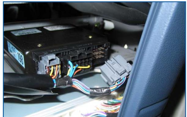
**12** Feed all the unconnected wires through the firewall boot in the upper passengers side of the firewall into the engine compartment. Some model trucks have firewall grommet near the accelerator pedal under the floor mat that can be used. Tape the firewall grommet to provide a water tight seal. Using the tie-straps provided secure the wiring harness and reinstall the dash panel.
