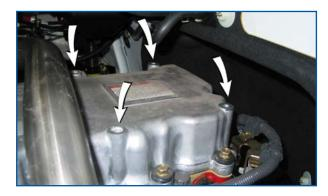
Using the 4 spacers provided, place one spacer on each of the 4 bosses. Install the 4 capscrews provided into the compressor bracket and place it over the spacers. Tighten the 4 capscrews to 15 lbs. ft. Connect the black compressor wire with the eye terminal to a good chassis ground, **DO NOT** attach it to the valve cover. A good ground location is the stud with nut on the firewall.
