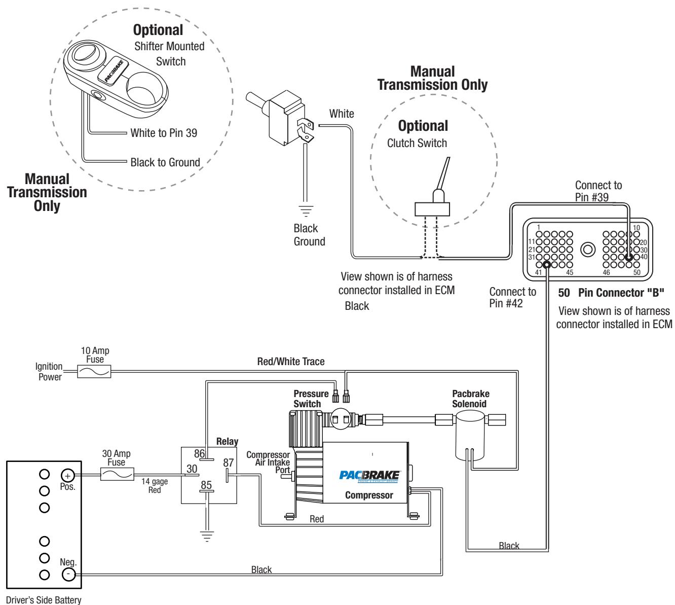
**NOTE: Compressor assemblies built prior to January 1 2005 are wired differently than shown in this schematic. Please visit our website to view previous schematic: [www.pacbrake.com](http://www.pacbrake.com).**
