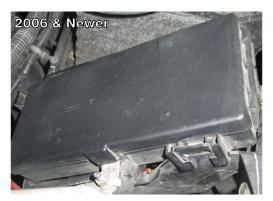
**NOTE:** Check the circuit with a volt meter for ignition power and 12 volts prior to attaching the "T" tap. Do not separate the connector as a fault code will be logged into the ECM. If you need to separate the connector, disconnect both battery leads. This will prevent the logging of a fault code in the ECM. Using the Blue "T" tap supplied, attach it to an ignition power source and then connect to the fuse harness supplied.
