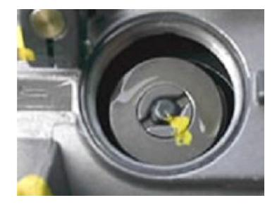
11 Using Vernier calipers measure the distance from the top of the governor stud to the top of the governor spring adjustment nut.
