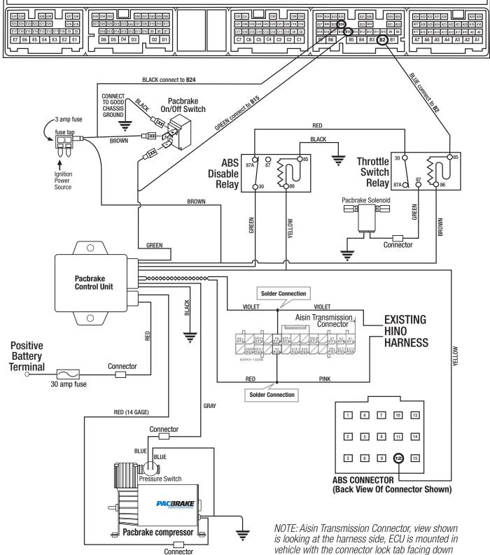
NOTE: Relays MUST be Diode Protected
