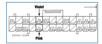
**11** Connect the VIOLET wire of the twisted pair to the VIOLET wire of the transmission connector. This connection must be soldered, and covered with the heat shrink provided.
