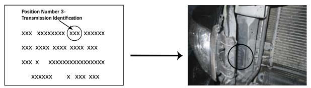
2 EQUIPMENT IDENTIFICATION STICKER - Check the 3<sup>rd</sup> description in left column (see illustration below) DG8 = Model 48RE - 4 Speed Automatic | DGP = Model 47RE - 4 Speed Automatic
