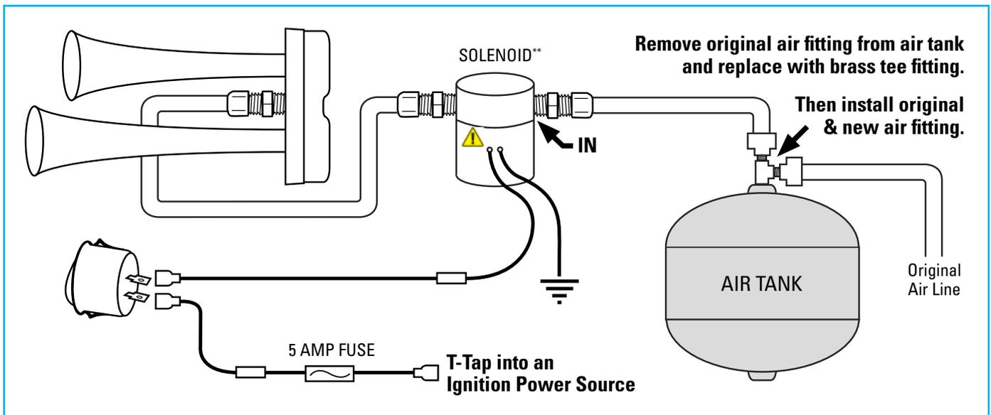
**⚠️ \*\*CAUTION: The solenoid included in 10314 / 10254 "Triple Train Horn" kits (Part No: C10613) are polarity-dependent: The BLACK wire must link to ground, the RED wire must link to power. Incorrect wiring will result in immediate failure of the solenoid.**
