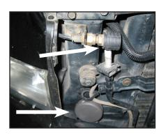
Make sure the nylon hose is cut square on each end and is pushed into the fittings until it clicks.
