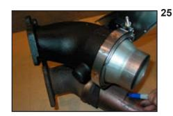
26 Install the 90 deg. fitting provided into the 1/8th NPT port of the air cylinder using thread sealant. At the turbo charger check the gasket surface for imperfections. If okay, install the new gasket and exhaust brake provided. Replace the 5 capscrews removed earlier with the supplied 12 point fasteners. Torque the capscrews to 110 in-lbs in a star pattern, then re-torque to 220 in-lbs in a star pattern.
