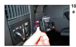
**10b** Install the dash switch and route the wires to the control unit. Secure the wires with the supplied tie-straps. At the control unit, locate the matching wire colors and connect using the supplied heat shrinkable red butt connectors. Once crimped, heat the connector to provide a water tight seal.
