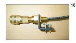
Make sure the nylon is cut square on each end and is pushed into the fittings until it clicks.
