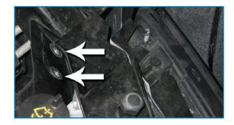
Remove the vacuum pump from the factory bracket, leaving the rubber isolators attached to the vacuum pump. Install the vacuum pump on to the Pacbrake supplied bracket as show in photo.
