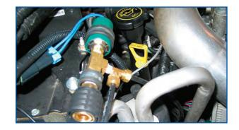
Route the Pacbrake connector with an orange and black wire to the solenoid valve mounted in the frame and connect.
