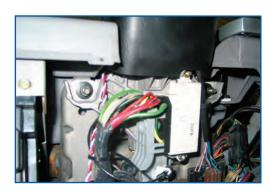
Locate the plastic cover plate on the drivers side of the firewall and remove. Drill a hole large enough to facilitate feeding the Pacbrake harness through. Feed all the remaining unconnected wires through the firewall into the engine compartment. Secure the Pacbrake harness neatly under the dash using the provided tie-straps. Re-install the firewall cover plate making sure it is clipped back into place.
