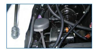
Install the fittings provided in the top of the air tank using thread sealant, as shown in the photo. Install the supplied ¼ NPT plug in the bottom of the tank. Choose a location on the outside of the frame to mount the air tank with the fasteners supplied (use existing holes in the frame if possible). Connect the airline from the pressure switch and air chuck assembly installed in step 15 to either of the two fittings at the top of the air tank.
