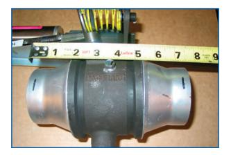
Select a location in the exhaust system that has sufficient clearance for installation and servicing of the exhaust brake. This location should be as close to the turbocharger as possible and away from dirt and road spray. Transfer the brake/adapter measurement, attained in step 2, to this location and mark the exhaust pipe. Remove the exhaust pipe and cut out the pre-marked section.
