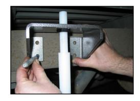
Using the slot in the lower bracket, slide the installation tool and upper bracket against the frame. Once the proper adjustment of the upper bracket is achieved, mark all 4 holes of the upper bracket to the frame. Remove the lower bracket, installation tool and upper bracket as an assembly from the vehicle. Mount the assembly onto the other side of the vehicle and mark the mounting holes. Make note of the position on the frame face, of the hole locations from side to side.
