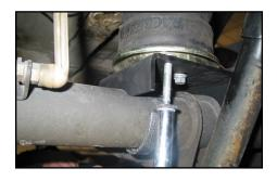
13 Ensure the alignment of the air spring has not changed.
