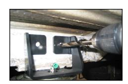
15 Insert two %"-16 x 4" bolts provided through the upper bracket and frame using the flat washers and nylock nuts.
