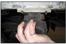
**6** Using a hammer, modify the small lip used to retain the jounce bumper.
