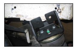
**8** Now install the frame spacer on top of the upper bracket.
