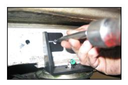
14 Check the inside of the frame for obstructions like electrical harnesses, fuel lines before drilling.
