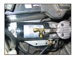
3 Connect the two air lines to the Tee fitting on the compressor (marked A), Connect the weather-pac connector of the wiring harness to the mating connector of the compressor. Install the blue nylon air line into the intake port of the compressor, (marked "B") located on the side of the crankcase.
