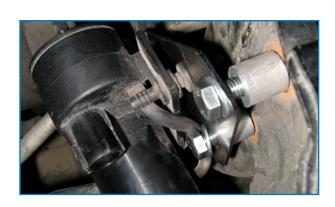
Locate the vacuum pump electrical connector disconnected in step 4. Cut the two wires 4" back from the connector. Using the lengths of BLACK and GREEN wire and the butt connectors provided, extend the harness to enable the connector to reach the new vacuum pump location. Once the butt connectors are crimped, heat the connectors to provide a moisture tight seal. Protect the harness with the conduit provided and secure with tie-straps.
