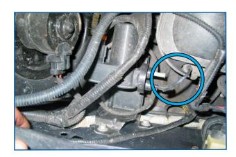
Remove the vacuum pump from the factory bracket, leaving the rubber isolators attached to the vacuum pump. Install the vacuum pump on to the supplied bracket as show in photo.
