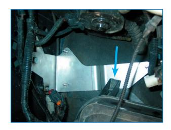
Note: The notch in the compressor bracket must be UNDER the vacuum reservoir foot.
