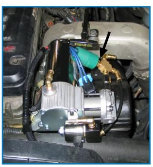
NOTE: The blind threaded port on the compressor head facing the front of the vehicle remains open.
