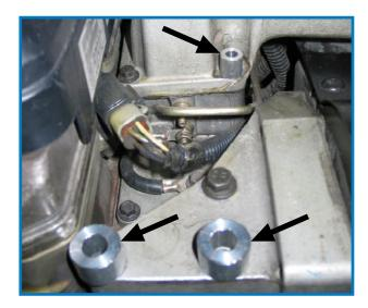
Install the compressor assembly over the 3 spacers.
