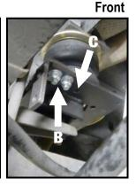
Insert a 10" carriage bolt into the unused square hole (C) from the top of the lower bracket.
