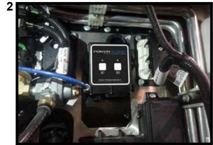
**3** | Connect the harness connector to the PowerGuard.
