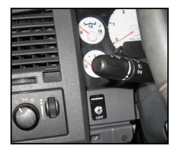
Remove the driver side knee panel to gain access to the base of the steering column.
