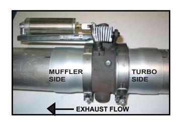
Continue routing the black nylon air line from the air solenoid, installed in step 14, to the inlet fitting of the exhaust brake air cylinder. Connect to the 90° air fitting.
