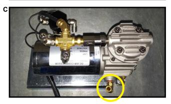
12 Apply thread sealant to all fittings installed.
