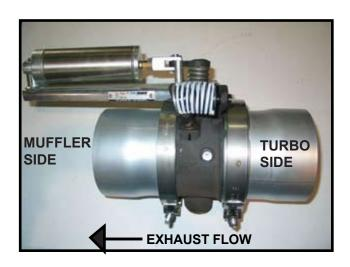
If removed, re-install the front section of pipe on the engine. Torque the turbo "V" clamp to the manufacturer's specifications.
