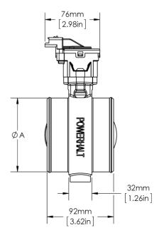
3.45 bar (gauge) [50 psig] -55°C to +175°C [-67°F to +347°F] -40°C to +120°C [-40°F to +248°F]
