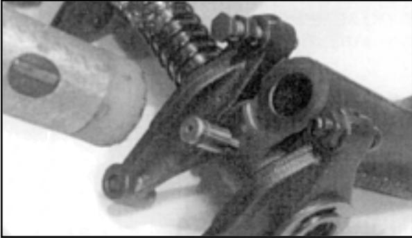
NOTE 1: This locating pin, as it is fitted into the milled groove on the undersurface of the housing, ensures proper alignment of the housing with the rocker arm shaft. CAUTION! The studs do not provide this alignment. Adverse wear to the master piston bore will result if you leave this important step out.
