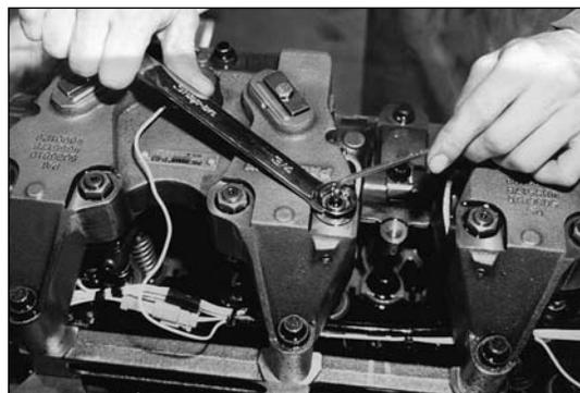
Double check all torques and wiring prior to reinstalling the valve cover. Use silicone sealant at front and rear bearing caps at valve cover installation. Torque valve cover bolts as per DDC service manual.
