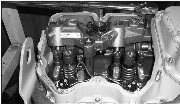
**NOTE: ALL MODELS.** The correct feeler gage must be inserted between the slave piston link and the exhaust rocker arm. DO NOT insert the gage between the crosshead and the foot of the adjusting screw, as improper lash will result and engine damage will occur.
