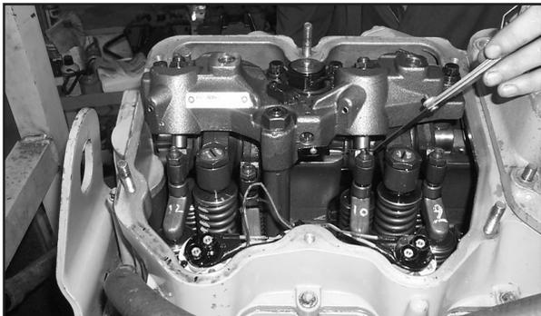
Turn in the adjusting screw beyond the contact point to squeeze out trapped oil. Back out the screw, then turn in again until a slight drag is felt on the feeler gage. Torque the locknut to **25 lbs.ft. (34 N•m)**. Repeat this procedure on the remaining cylinders with closed exhaust valves. Rotate the crankshaft to the next valve set position to adjust the remaining cylinders. Double check torque on the locknuts.
