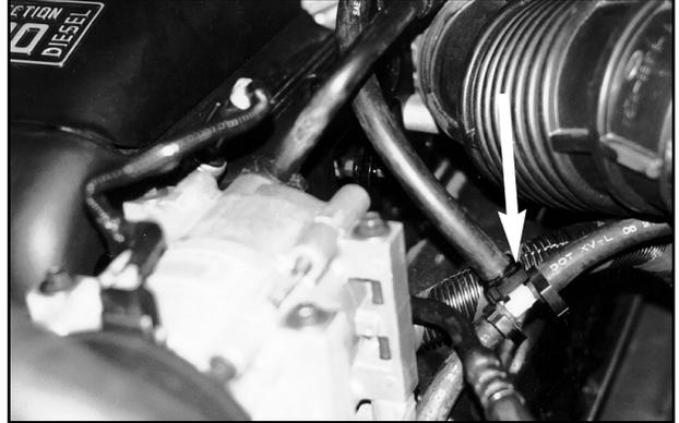
**IMPORTANT: Double check all fittings, clamps and connections, including the main vacuum connection. Ensure the hoses at the vacuum cylinder have been secured as far away from the exhaust components as possible. Leaks could cause partial loss of braking.**
