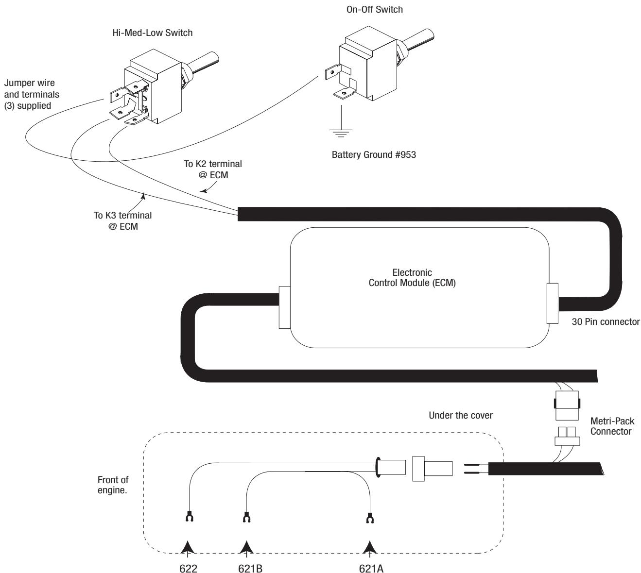
**The Metri-Pac connector located above the starter is the same as previous 1999 engines.
