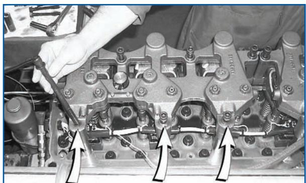
**Note: Ensure that each master piston link is located over its rocker arm socket.**
