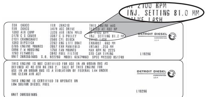
These new 2000 model year engines are built starting late December 1999 and differ from the 1999 model year engine by the elimination of the engine brake's dedicated roller on the injector rocker arm. The 2000 model year engine has a machined pocket in the injector rocker arm to replace the roller. Installing the incorrect engine brake will cause engine and engine brake failure.
