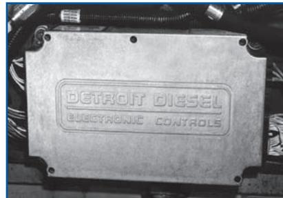
**NOTE: Some DDEC IV engines may not have the ECM programmed for engine braking. This may be verified using a Diagnostic Data Reader. If any of the ECM input switches; K2, K3, S3 or T3 read NONE, then the vehicle should be taken to a DDC dealer to have these switches enabled.**
