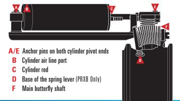
ONCE ALL POINTS HAVE BEEN LUBRICATED, CYCLE THE EXHAUST BRAKE FITHER FLECTRONICALLY OR MANUALLY TO WORK IN THE LUBRICANT.
