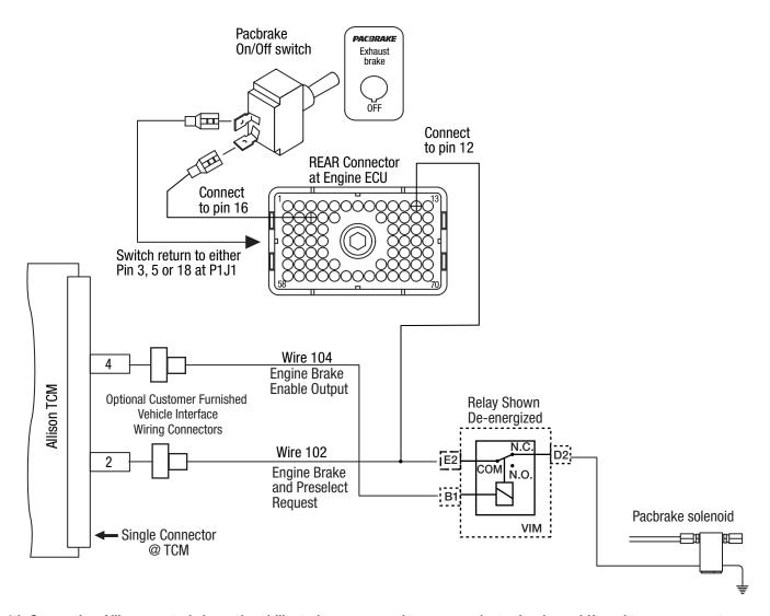
4th Generation Allison controls have the ability to be programed to communicate the downshift and torque converter unlock features over the Data-link J1939. Doing so eliminates the need to hard wire the exhaust brake circuit to the transmission ECU, the exhaust brake circuit only needs to be hard wired with the engine ECU. Consult your closest Caterpillar or Allison dealer for a quote, Pacbrake offers an interface kit C13074 if hard wiring is your preference.
