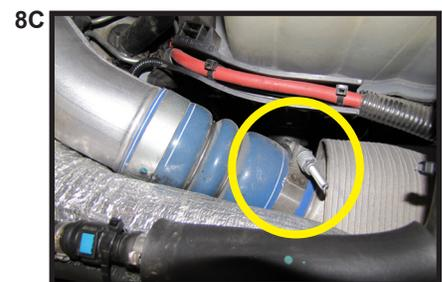
**9** Once the pipe is removed, mark each end of the pipe with the letters 'A' and 'B'. 'A' will be your turbo side, and 'B' will be the CAC side.
